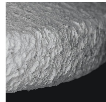
Microscopic observation (x500) of implant surface with Anthogyr BCP surface treatment
